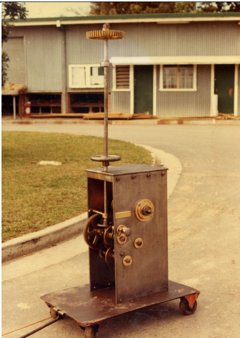
Figure 23. The Optic turning mechanism prior to installation at the museum
