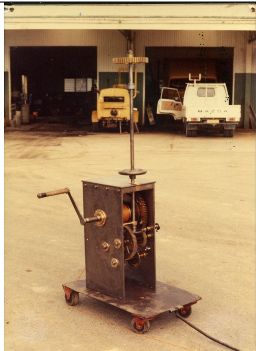
Figure 24. The Optic turning mechanism prior to installation at the museum
